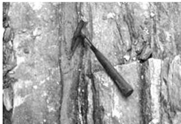
Figure 16. Vertical layer of weathered biotite schist (in the middle of the photo) within crystalline gneiss.
