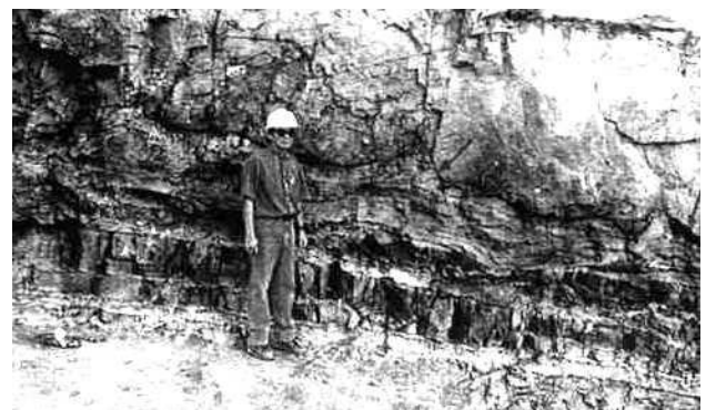
Figure 7. Detail of the siltstone intercalations in the sandstone, corresponding to a weak layer.
