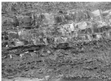
Figure 5. Siltstone intercalations in sandstone, at the Castrovido dam foundation in Spain (Alonso, 2011)
